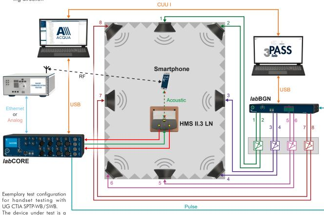
smartphone in handheld hands-free mode. A radio communication tester establishes the RF connection to the phone, HMS II.3 LN simulates its user
