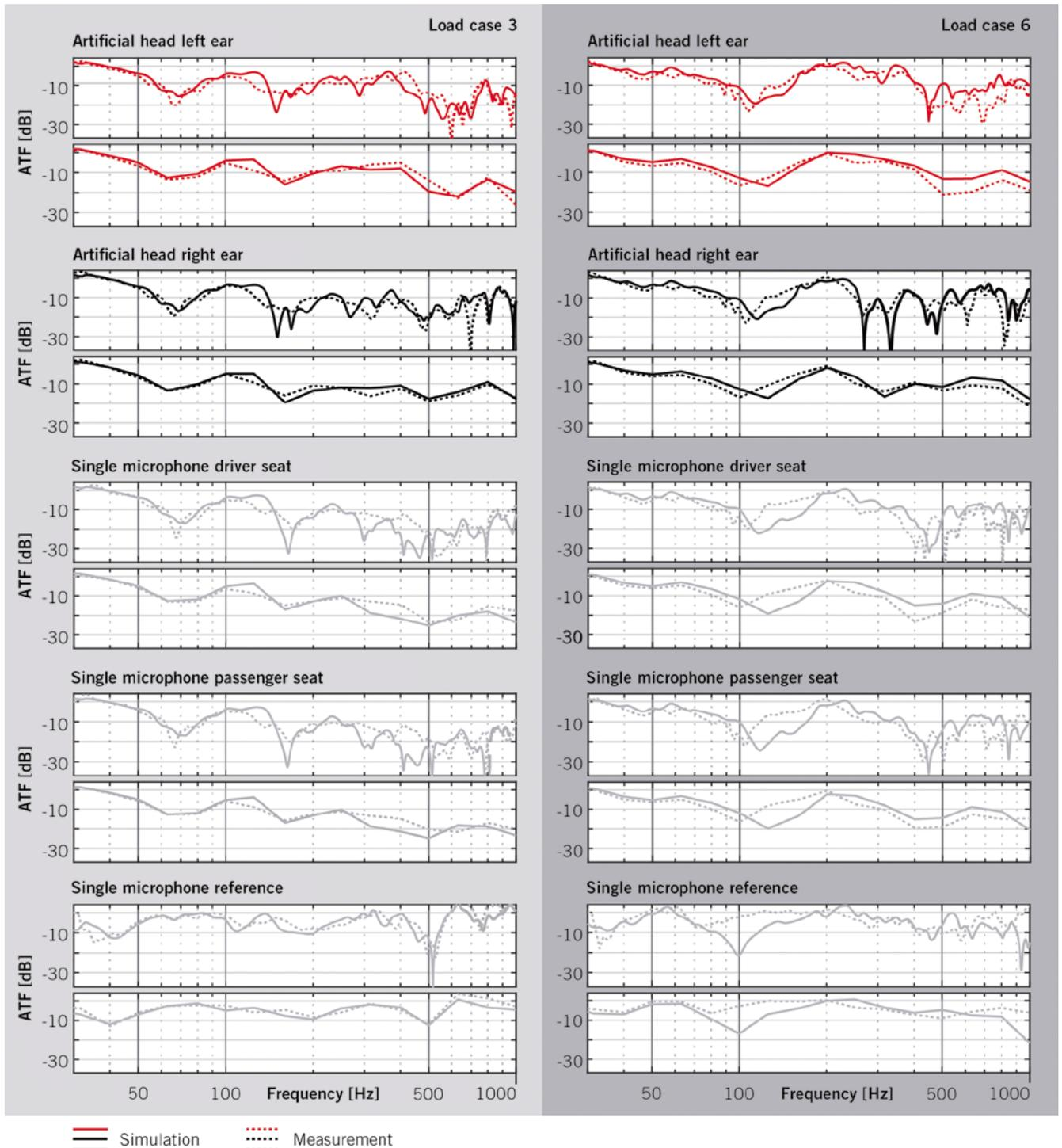
**FIGURE 5** Comparison of measured and simulated Acoustic Transfer Functions (ATFs) in the narrow band and third octave band for load case 3 (left) and load case 6 (right) © Head acoustics GmbH | Dr. Ing. h.c. F. Porsche AG
