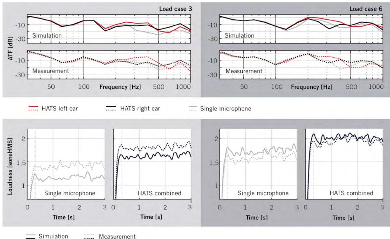
**FIGURE 6** Top: Comparison of the sound pressure at the single microphone to the artificial head's ears for simulation and measurement in the third-octave band, load case 3 (left) and load case 6 (right). Bottom: Loudness rating comparison according to ECMA 418-2 between simulation and measurement for the single microphone and combined for the artificial head, load case 3 (left), and load case 6 (right) © Head acoustics GmbH | Dr. Ing. h.c. F. Porsche AG
