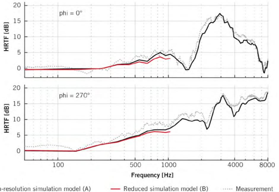
**FIGURE 3** Reduced FE model of the Head and Torso Simulator and HRTFs of the right ear for the directions 0°/front and 270°/right: comparison of measurement, high-resolution, and reduced simulation model (© Head acoustics GmbH)
