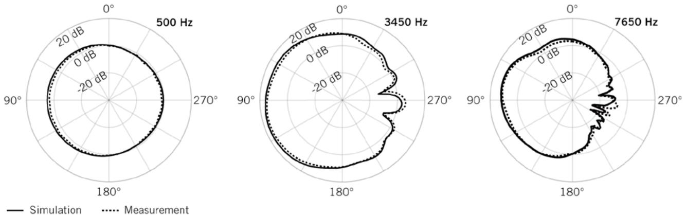
**FIGURE 2** Comparison of measurement- and simulation-generated HRTFs in the polar diagram in the horizontal plane for the left ear for 500 Hz, 3450 Hz, and 7650 Hz (f.l.t.r.) (© Head acoustics GmbH)
