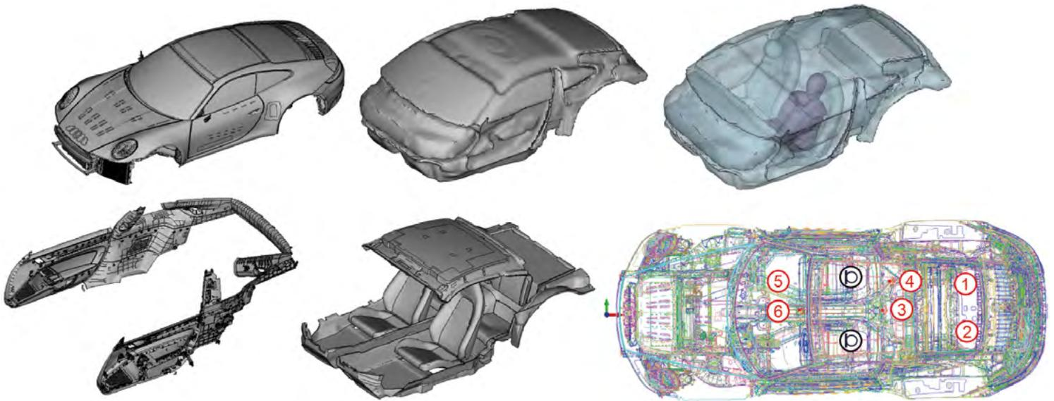
**FIGURE 4** Representation of the simulation model consisting of structural model (top left), interior cavity (top center and right with artificial head), interior paneling parts (bottom left), and trim (bottom center). The excitation positions numbered according to the load case are marked in red, and the measurement positions are marked in black (bottom right) (© Dr. Ing. h.c. F. Porsche AG)
