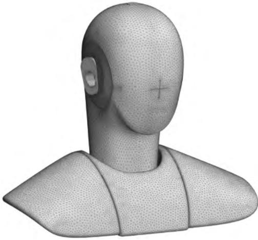
**FIGURE 1** High-resolution finite element model of the HMS IV (© Head acoustics GmbH)
