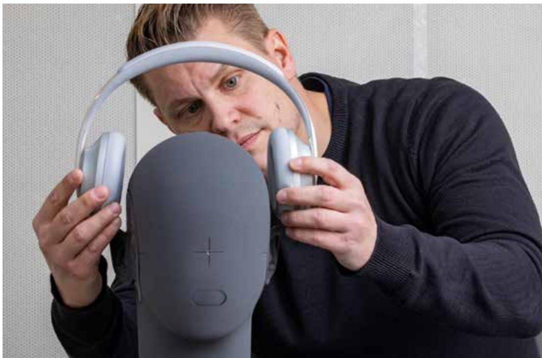
Realistic headset testing with human-like pinnae
