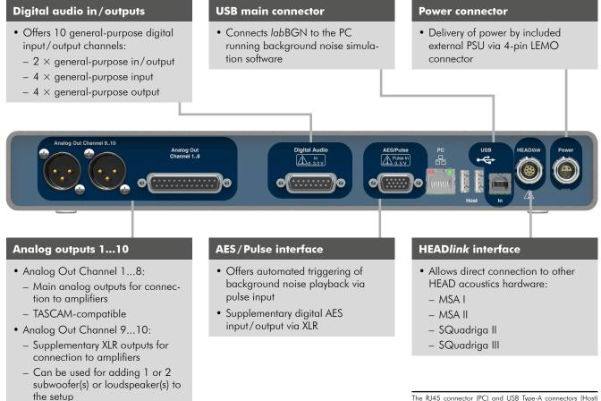
The RJ45 connector (PC) and USB Type-A connectors (Host) currently are only for internal use. The USB Type-A connectors (Host) can be used for charging/powering USB devices.
