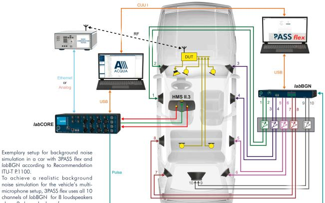
ITU-T P.1100. To achieve a realistic background noise simulation for the vehicle's multi-
