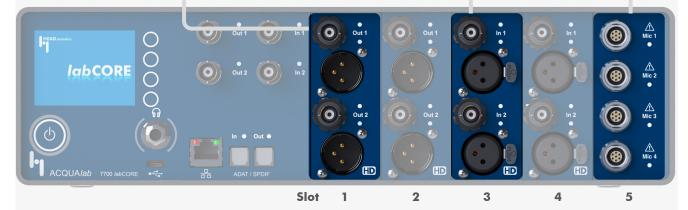
The five extension slots at the front are designated for the most common extension boards coreOUT-A2 and coreIN-Mic4. A total of two coreIN-A2, two coreOUT-A2 and one coreIN-Mic4 can be installed, providing twelve high-precision low-noise analog channels for arbitrary precision measurements: four inputs, for outputs and four microphone inputs.
