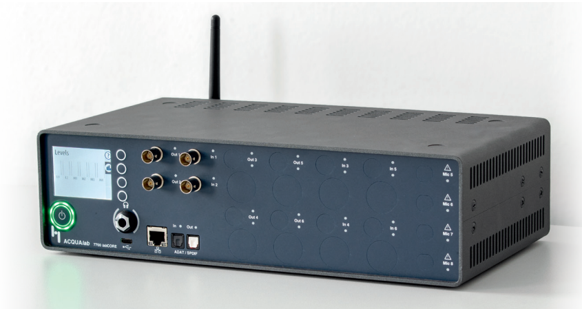
labCORE in basic configuration (no extension boards) with coreBT module and installed RF antenna
