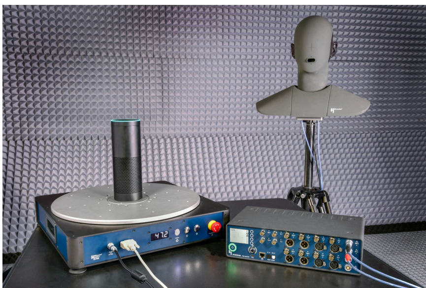
Exemplary measurement configuration with smart speaker on HRT I, HMS II.3 and labCORE
