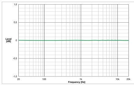
Typical frequency response of HIB I (all inputs/outputs)
