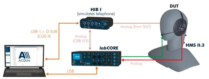
Setup with HIB I as the headset part of a telephone to test a headset
