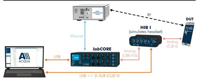
Setup with HIB I as a headset to test a mobile phone
