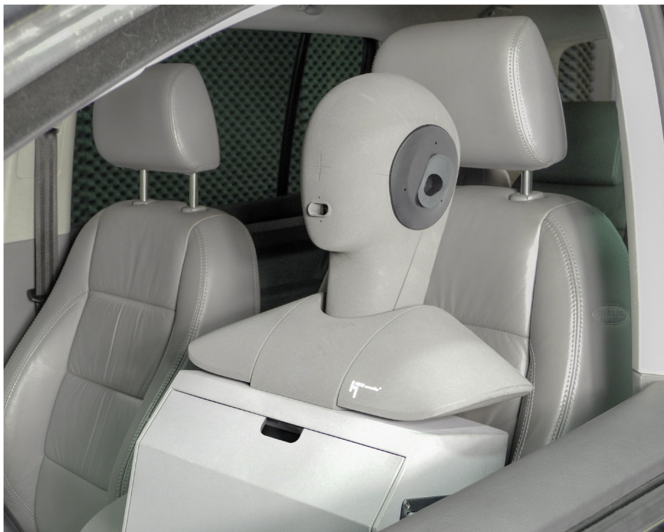
HMS II.6 on torso box HTB VI in a typical in-car hands-free communication test scenario
