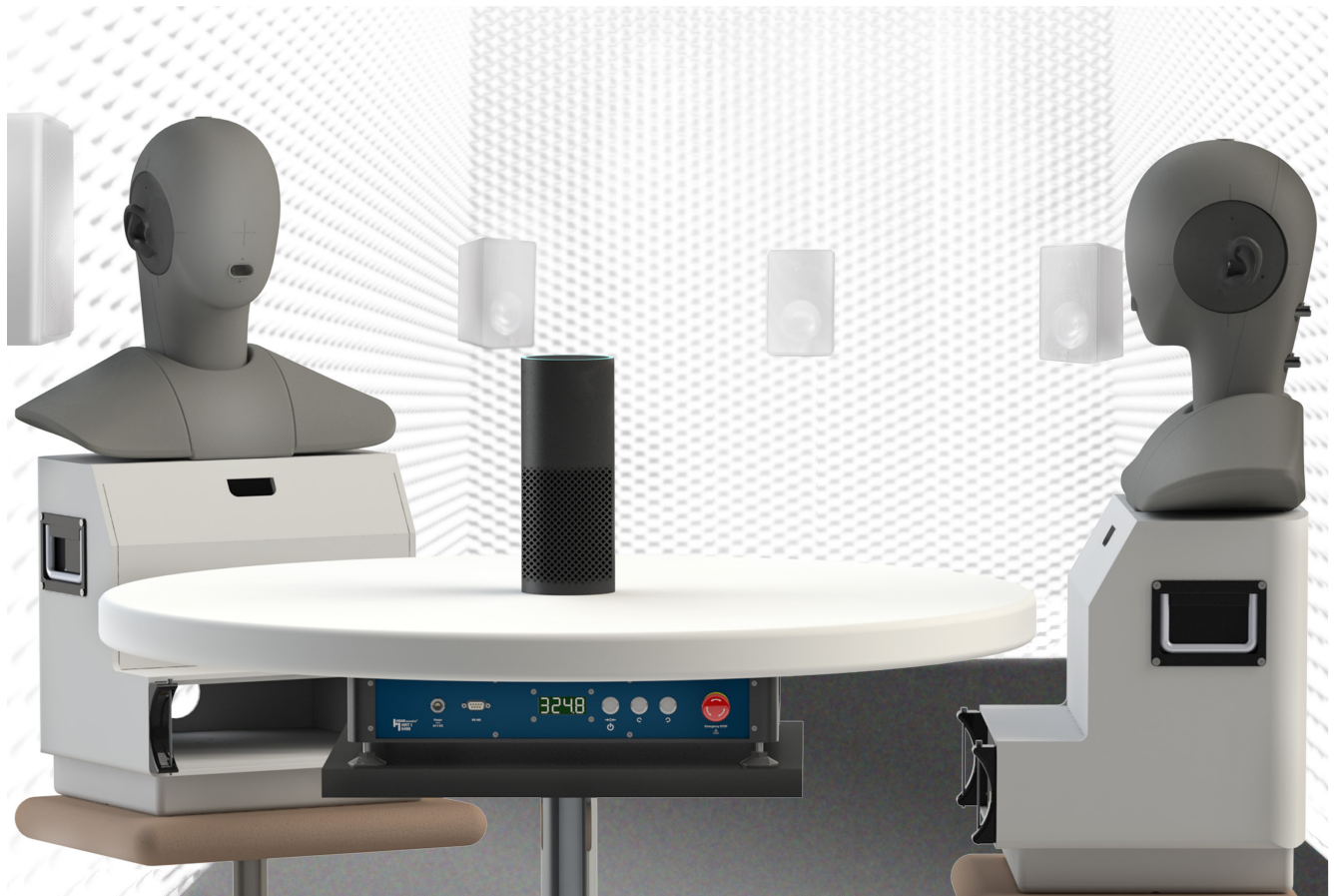
Exemplary application: HMS II.3 (on the left), HMS II.5 (on the right) and a smart speaker on HRT-I in a multi-talk test scenario
