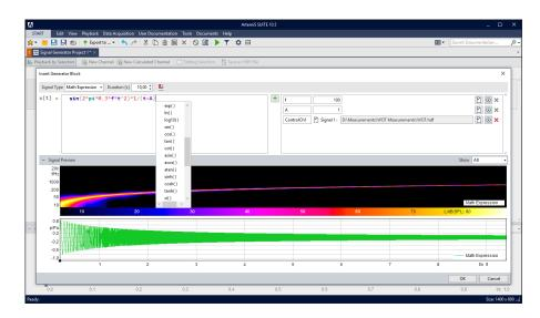
Example of a mathematical formula in a Signal Generator Project: The time-domain curve and an FFT vs. time analysis are displayed immediately.
