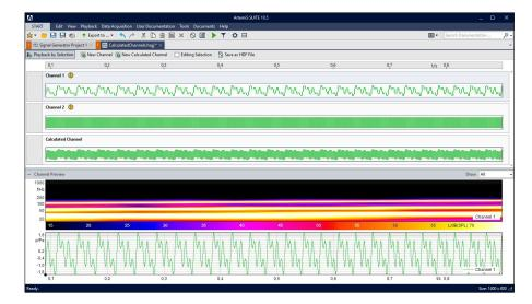
With the Calculated Channels function, users can switch between several source channels to evaluate the effects in the channel preview immediately.
