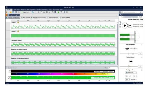
In order to save intermediate results, the snapshot function can be used to create an image of the respective channel as new block in a new channel.
