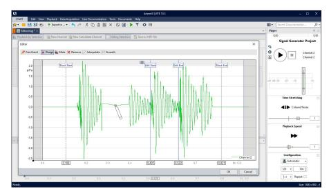
In the Editor diagram, all channels can be post processed manually. Using the Free Hand Mode, users can redraw the whole curve graphically with a pen.
