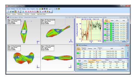
The ME'scope $VES^{TM}$  analysis software allows the creation of an animated model of the measured transfer functions.
