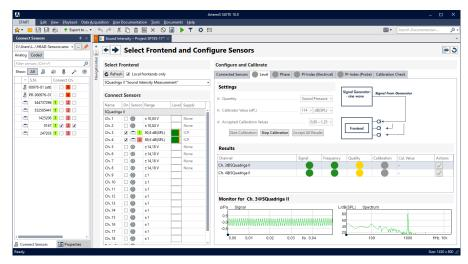
During level calibration, the current progress and the status of all channels currently handled by the calibration are displayed. To the right of the settings, a setup scheme facilitates the creation of a measurement setup suitable for channel calibration.
