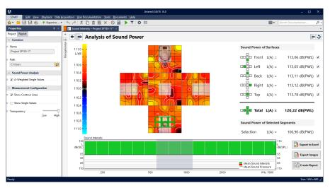
To calculate the sound power, users can select the pages that should contribute to the overall result. The butterfly diagram shows the averaged sound intensities of all selected segments in the 2D view.
