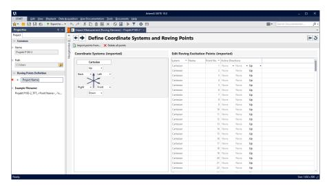
The configuration and orientation of triaxial acceleration sensors is done quickly and safely thanks to easy handling and the use of common names.
