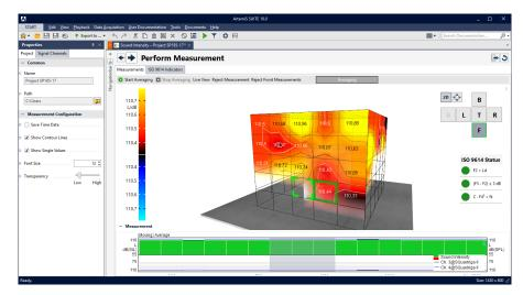
Easily identifiable for the user during the measurement, the next points to be measured and the corresponding face of the measurement area are highlighted with a green frame. Below that, a butterfly diagram shows the moving averages of the sound intensity as columns and the signal levels of all active, connected channels as curves.
