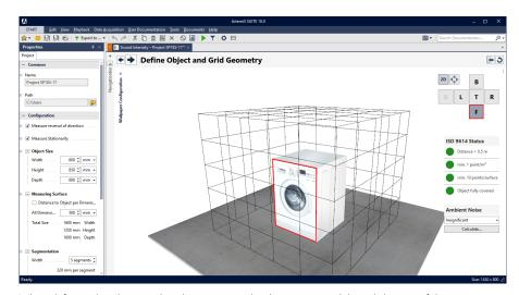
When defining the object and grid geometries, the dimensions and the subdivision of the measurement area surrounding the test object can be specified very easily. Images of the test object can be mapped onto the faces of the 3D box representing the object.
