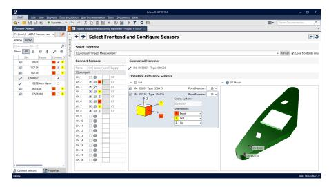
The front-end and sensor configuration can be used to select the front end, to connect the desired sensors and to specify the orientation of the reference sensors.
