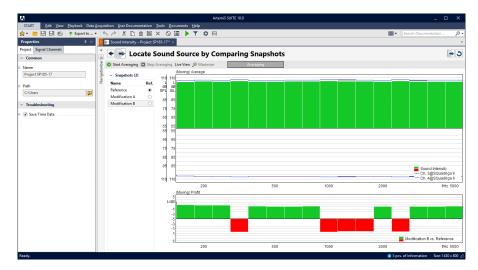
Using the quick diagnostics method, butterfly diagrams allow users to perform and save real-time comparison measurements or localization measurements. In addition to the sound intensity and level data, the underlying time signals can also be saved.
