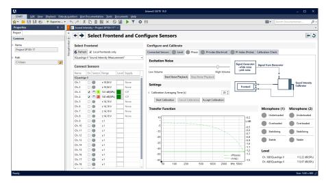
For the phase calibration of a PP probe, it is also possible to use noise playback via an internal or external sound card (e.g. the *labO2* equalizer), where the noise volume can be adjusted with a slider.
