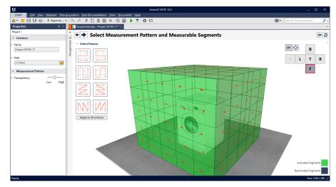
When specifying the pattern based on which the individual segments are to be processed during the measurement, partial areas can be excluded from the measurement.
