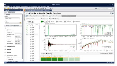
The measurement window provides four different diagrams, showing the time domain signal, the time domain signals of all specified reference points, the coherence, and the transfer function.
