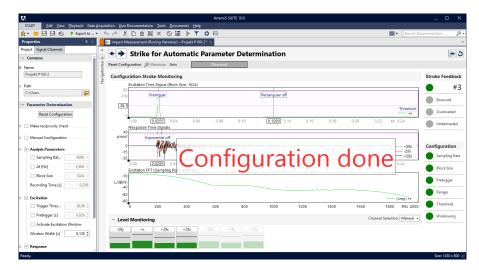
During the automated acquisition of the measurement parameters, users get both acoustic and visual feedback (via colored LED icons) as well as information as to whether the strike was double, too strong or too weak.
