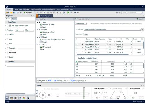
In semi-automatic design mode, the results of jury tests are accounted for automatically in order to map them on the measured analysis results from the sequence area in the best possible way.
