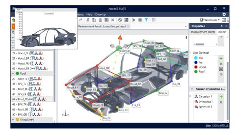
Using the import, the number of model points of complex CAD models can be reduced. Imported Measurement Point Libraries offer different display options: full surface, wireframe, or transparent. Measurement point numbers, names, lines etc. can be shown or hidden.
