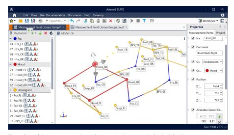
The surface of the Measurement Point Library is clearly structured. On the left, all measurement points defined in the Measurement Point Library are listed with their mandatory number. The properties allow various adjustments, such as sensor orientation, to be controlled and corrected as needed.
