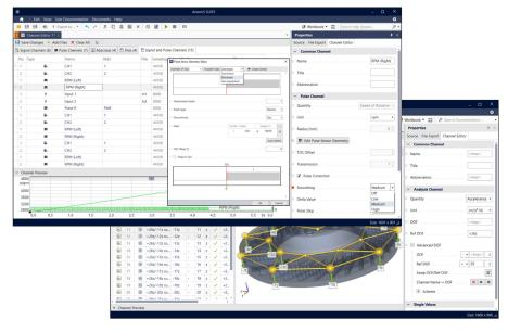
The Channel Editor offers a detailed overview of all channel properties and it also allows to change most of them. Users can perform the desired changes of the channel properties either for individual channels directly in the Channel Editor or via the additionally opened Properties tool window.
