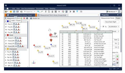
HEAD acoustics provides guidance concerning the structure of how the measurement points are defined with Excel. Typically, five to five hundred measurement points are captured.
