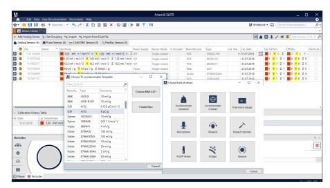
The Sensor Library shows the respective sensor type as an icon and the available sensor parameters in a clearly arranged layout and also notifies the user of problematic settings.
