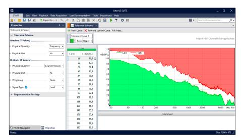
All curves contained in a Tolerance Scheme are displayed in the diagram with the full functionality available, e.g., zoom, various cursor modes, and fill areas.
