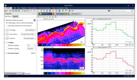
The Data Viewer is used for the customized display of analysis results. The Result Routing allows the criteria for the layout of the individual diagrams to be selected.
