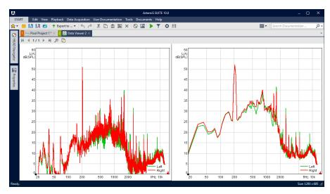
For this low-frequency tonal sound, which hardly changes over time, the averaged VFR analysis (left diagram) is especially well suited. Unlike the averaged FFT analysis (shown in the right diagram), the VFR analysis has a better spectral resolution in the low-frequency range and shows the frequency of the hooting sound with a very narrow peak at 205 Hz.
