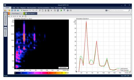
The modulation depth and the modulation frequency can be detected by using several modulation analysis.
