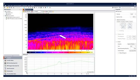
In addition to the methods of automatic RPM determination, manual drawing with the pen tool is available. Users can completely draw a new curve and save the result as a new RPM curve.
