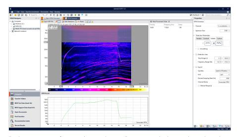
For the measurement of rotating objects such as small engines or turbochargers, the mechanical acquisition of the revolution speed often turns out to be tricky or it is not possible at all. The RPM Generator allows it to extract this information from the normal measurement signals.
