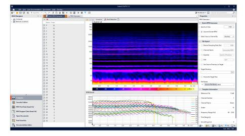
The order determined in each case is displayed in the corresponding column of the table. In the FFT vs. time diagram, the estimated model curve is displayed for control purposes. The result converted out of the frequency is available as RPM vs. Time in the lower diagram.
