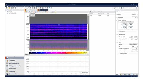
To make it easier for users to process a large number of similar measurements, the RPM Generator can be used to create a corresponding template, which can then be applied to the complete data set using the Batch RPM Generator.
