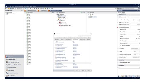
RPM Generator templates can be embedded into an Automation Project as a normal processing step. Via HEAD Navigator, Automation Projects with RPM generation can also be applied to entire folders with a large number of similar files.
