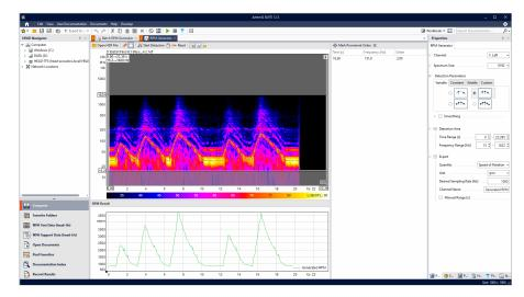
Depending on the measurement, the settings can be selected variable, constant or volatile. Variable is suited for run-ups, coast downs, and combined run-ups/coast downs of combustion engines, as well as for the determination of frequency fluctuations of electrical auxiliary drives.
