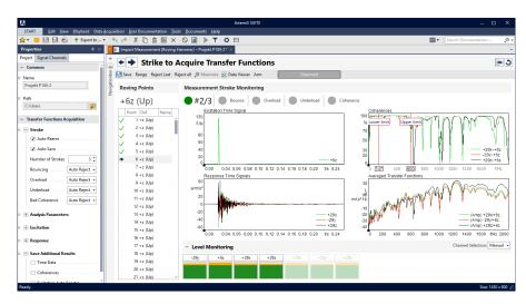
The measurement window provides four different diagrams, showing the time domain signal of the excitation, the time domain signals of all specified reference points, the coherence, and the transfer function.
