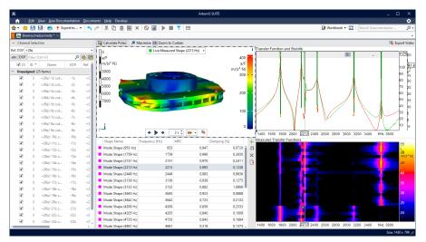
Using the Modal Analysis Project, the analysis of the recorded data can be performed by means of live coupling already during the measurement. Alternatively, impact measurements that have already been performed can also be analyzed offline there. Within the analysis, all necessary information are clearly displayed via various diagrams and animations.
