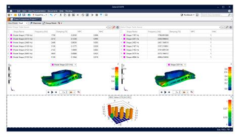
The Shape Comparison Project determines the MAC (Modal Assurance Criterion) value and provides information about the similarity of deflection shapes. This information can be used, for example, to assess the quality of a simulation.
