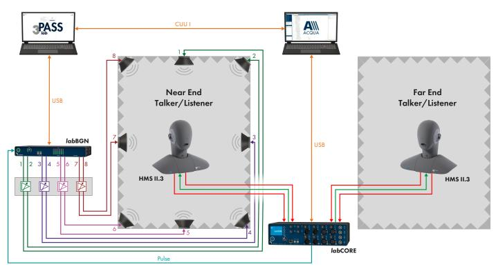
A generic setup for Measurements with HQS-Ac2Ac. At each end of the transmission path, a HMS simulates the DUT's user. Both are situated in an acoustically separated anechoic environment. They are connected to one common labCORE hardware platform, binaurally as well as with their artificial mouth. Both support far-from-the-ear as well as close-to-the-ear DUTs, therefore the
