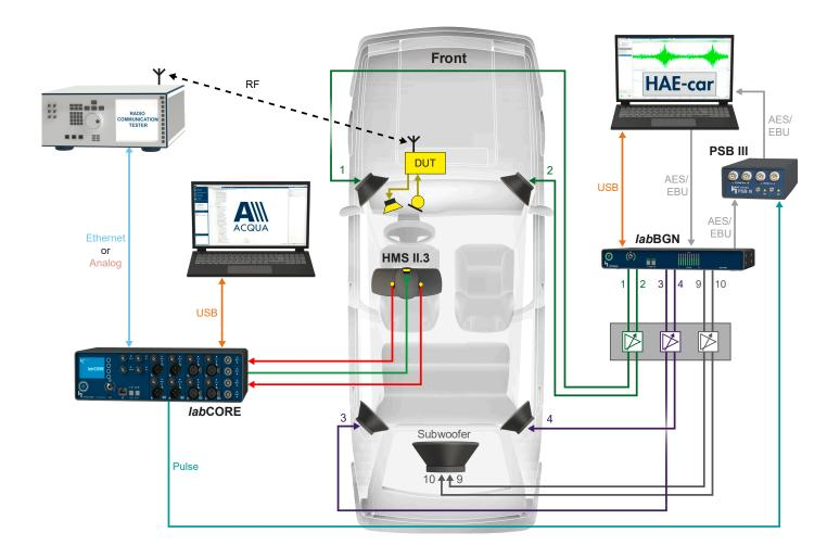
This standard requires an artificial head according to ITU-T P.58. When equalized, HMS II.6 & HMS II.7 can be treated as P.58-compliant for farfield measurement purposes.
