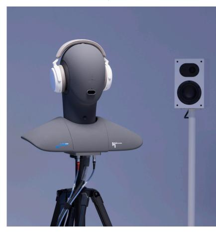
performance or the performance of voice call communication of the device under test. A second artificial head or an external loudspeaker can play back speech signals as concurrent talker with or without the presence of background noise.
