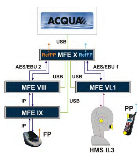
Example configuration: CAT-iq $^{\text{TM}}$  acoustic measurements with analysis system ACQUA, artificial head HMS II.3, front ends MFE VI.1, MFE VIII, MFE IX and MFE X.
