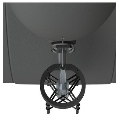
9. Remove the MRP pointer and the lip ring carefully. Do not change the position of the microphone anymore.
