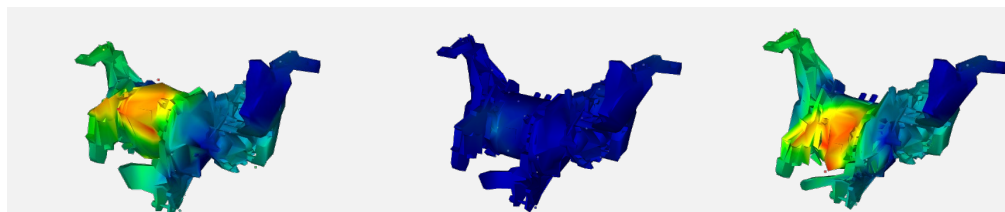
Vibration modes of a powertrain
