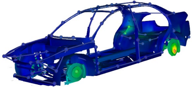
Visualizing operational deflection shapes easily in ArtemiS SUITE
