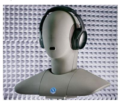
HQS-ANC-Headset is the new test suite from HEAD acoustics' for the use with the communication quality analysis system ACQUA. The measurements enable manufacturers to test and further develop state-of-the-art (ANC) headphones and headsets.
