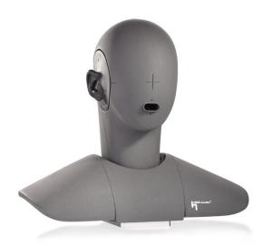
Ear simulators with highly sensitive microphones assure a very low inherent noise of 16 dB<sub>SPL</sub>(A) of the binaural artificial head measurement system HMS II.3-LN.
