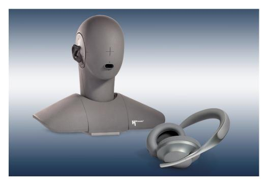
Due to the very low inherent noise, HMS II.3-LN is ideally suited to assess the quality of ANC headsets and headphones as well as other close to the ear audio and telecommunication equipment
