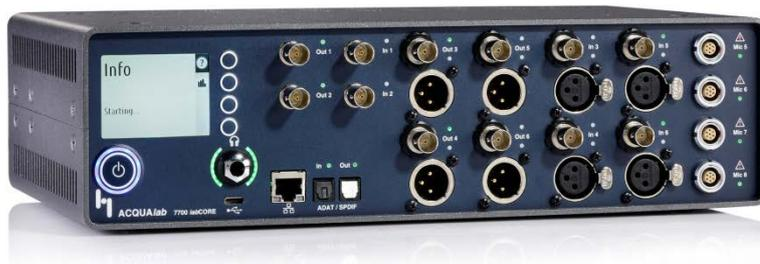
*labCORE* is the modular multi-channel front end for precise and efficient voice and audio quality measurements
