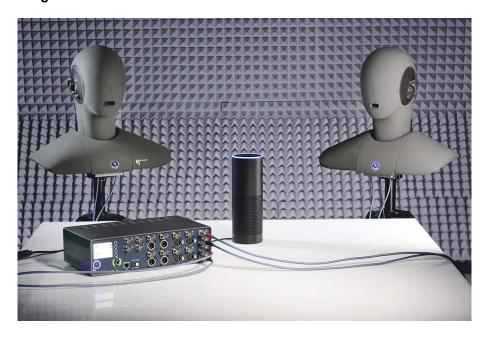
VoCAS supports the modular multi-channel front end *lab*CORE. This extends the possibilities for evaluating voice control system in e.g. smart speakers.
