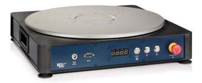
HRT I is a high-precision turntable for automated, orientation-dependent acoustic measurements
