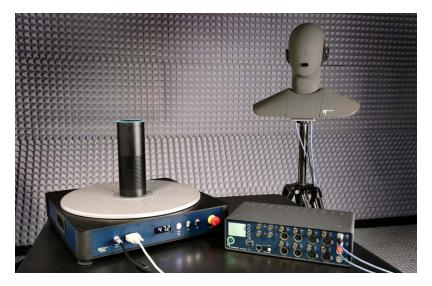
Testing e.g. smart speaker with *lab*CORE, HRT I and artificial head measurement system HMS II.3
