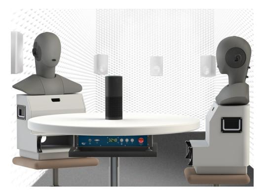
For simulating the different positions of moving speakers, directivity measurements are implemented in HQS-SmartHome.
