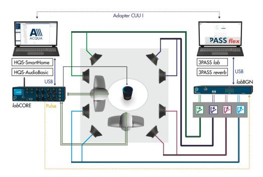
This exemplary measurement setup of HQS-SmartHome consists of two artificial head measurement systems positioned around the device under test, ACQUA including HQS-SmartHome and further software and hardware components.
