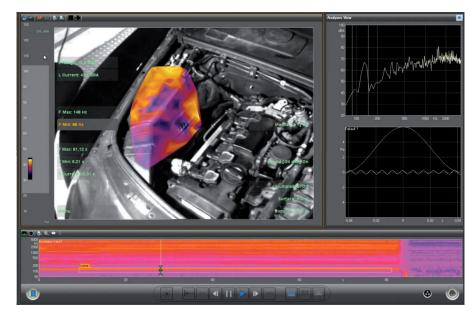
The near-field HEAD VISOR Probe is excellently suited for the examination of low frequencies, such as the 150 Hz humming of this intake filter.
