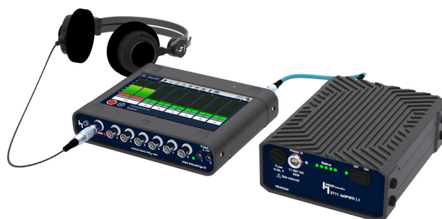
Power supply using a labPWR I.1 Power Box
