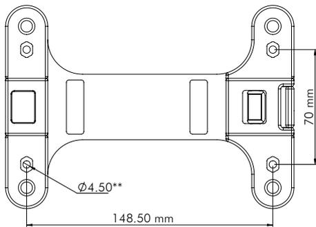
\*\* The 4.5 mm through holes can be used to additionally fasten the labMA Mount Adapters
