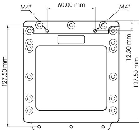
\* The M4 threads can be used to additionally fasten the *labCP* Screw Fasteners
