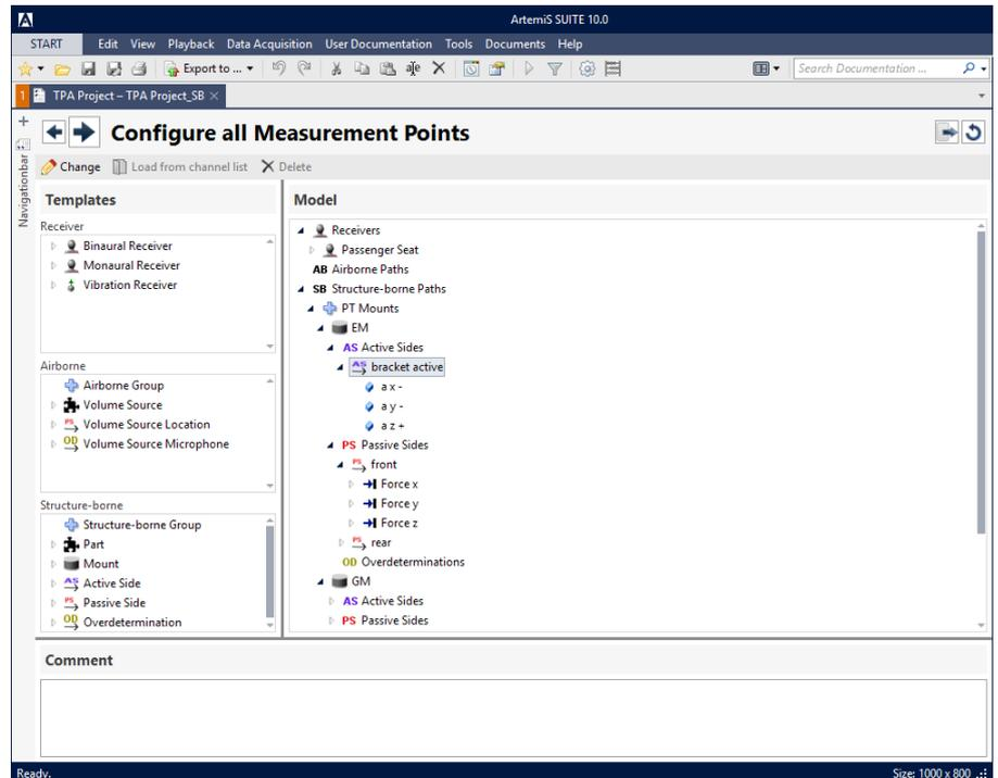
For creating a TPA project with ArtemiS SUITE, the convenient tree structure facilitates the procedure. Via drag and drop, the templates can be moved from the left side into the desired composition.
