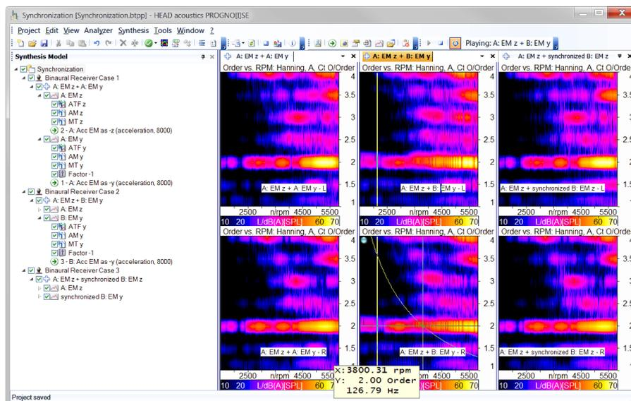
Reinforcements and cancellations (in the 2nd motor order), caused by a superposition of non-synchronous input data, can be prevented by synchronizing via order synthesis.
