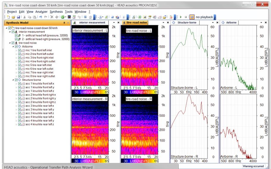
The OTPA Wizard creates a PROGNO[I]SE model that allows, for example, tire noise of a vehicle to be synthesized.
