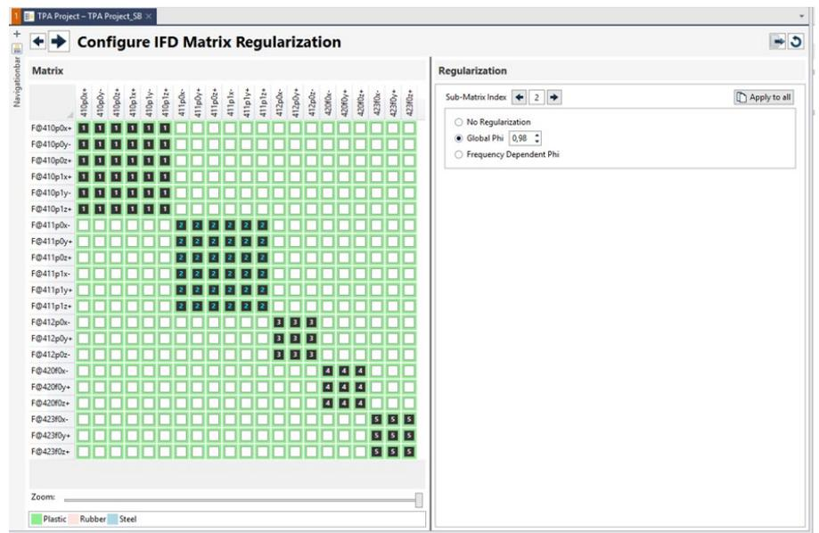
In order to prevent that small measurement errors in the input data lead to an overestimation of path contributions resulting in case of badly conditioned matrices, matrix inversion with frequency-dependent regularization are used.
