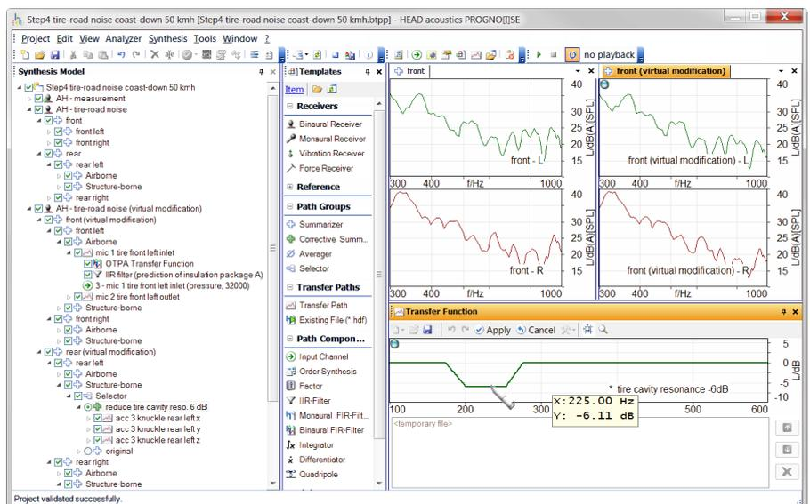
Even large models can be managed easily with PROGNO[I]SE. Various tools are available for editing, e.g., for smoothing and inverting of transfer functions.
