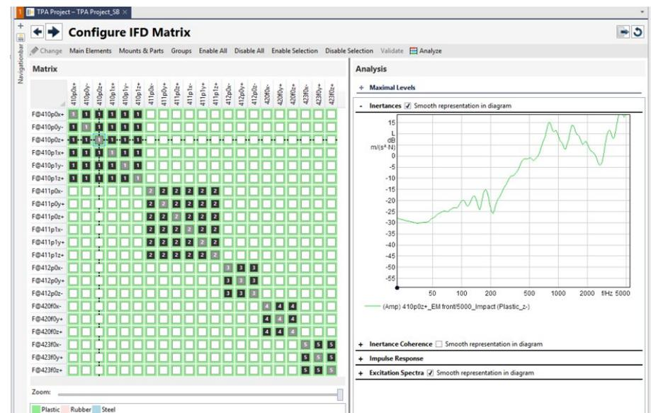
Immediately, the bar display and various diagrams allows the user to check the properties of the impact measurements visually. Subsystems can be independently considered. For that, the associated submatrices are calculated individually and configured independently from each other.
