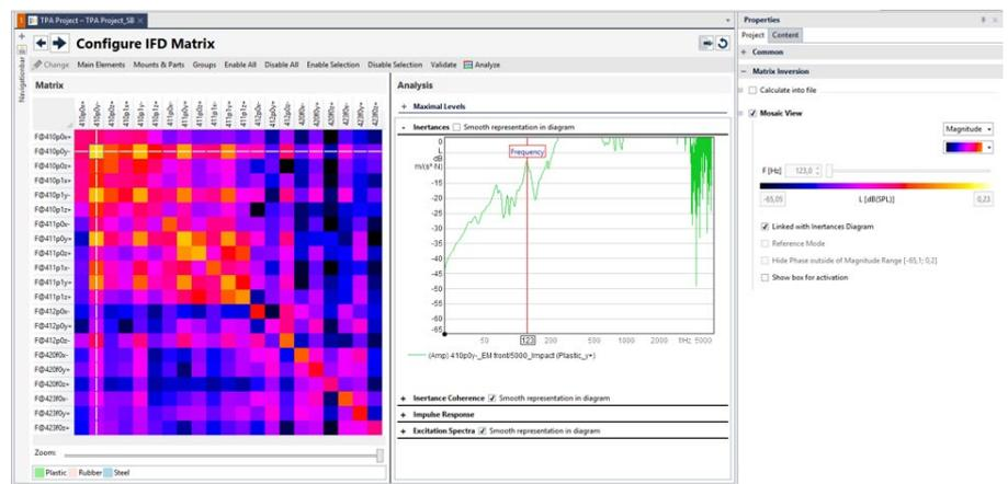
The Mosaic View visualizes the magnitude or the phase of the transfer functions in form of a frequency-dependent, color-coded matrix. This makes it easier for users to gain a profound understanding of systems and provides an aid to decision-making, whether coupling between subsystems must be considered or can be neglected.
