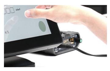
The original sound spectrum and the spatial distribution of the sound field can be exactly reproduced using the labP2 playback module and headphones from HEAD acoustics.
