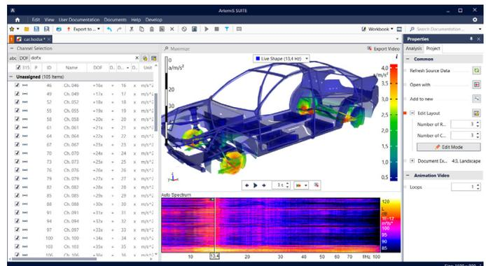
*Channel Selection: The Channel Selection allows filtering the channel list via the input field. Selected channels can be activated or deactivated by means of multiple selection. In addition, the column headings can be used for sorting.*
