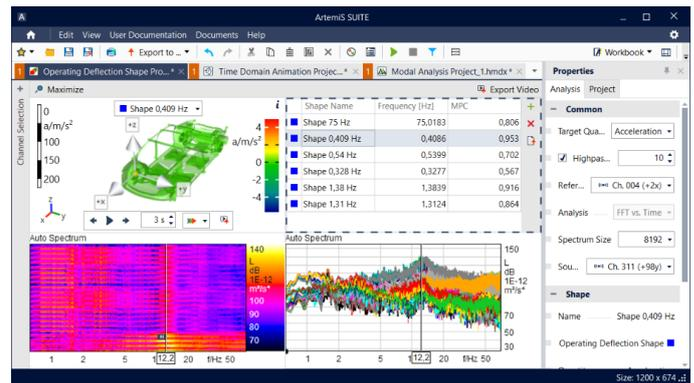
*Operating concept: Users can keep an eye on all operating, analysis, and animation sections while evaluating the data, which greatly increases the usability. Optionally, users can maximize one section at a time.*
