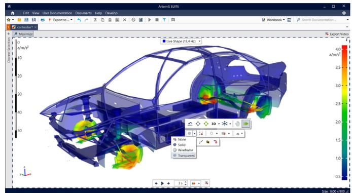
The deflection of the shape can be adjusted using both scales, movement on the left side and color on the right side. The animation speed can be adjusted via the loop duration input field.
