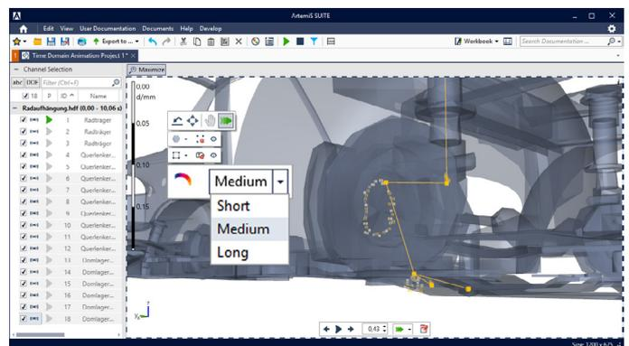
During the animation, the positions of the measurement points are altered according to the scale on the left. By means of the Trace Tool, the course of the movement of each measurement point can be clearly visualized in the form of a fading trace.
