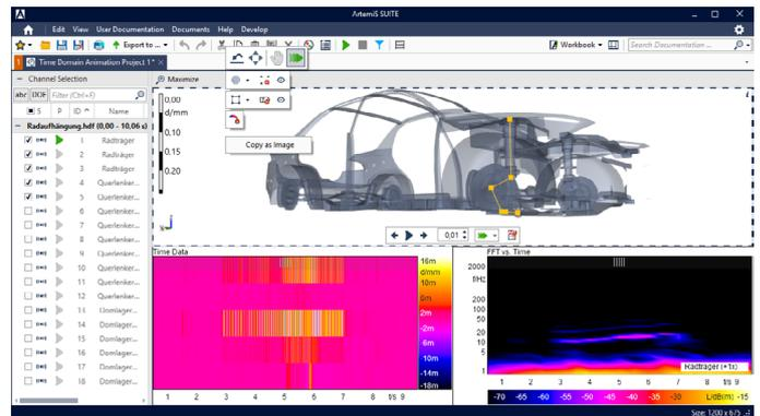
The work area of the TDA Project is initially divided into different sections: Channel Selection, Animation, and the analysis area with the two diagrams time data. Analog to the ODS Project, users may customize the layout from the analysis.
