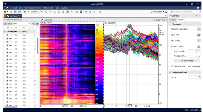
As in the auto spectra, the frequency to be used for the animation can also be determined in the 2D diagram (airborne channels) by double-clicking. Here, the Value Cursor can be moved horizontally with the mouse, too.
