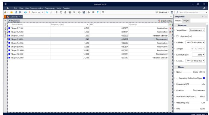
The MPC index of each shape evaluates the collinearity of the modal phases of all channels. Small phase differences between the channels or a rotation by 180° result in good values of up to 1. The greater the phase differences, the more this value tends to 0.
