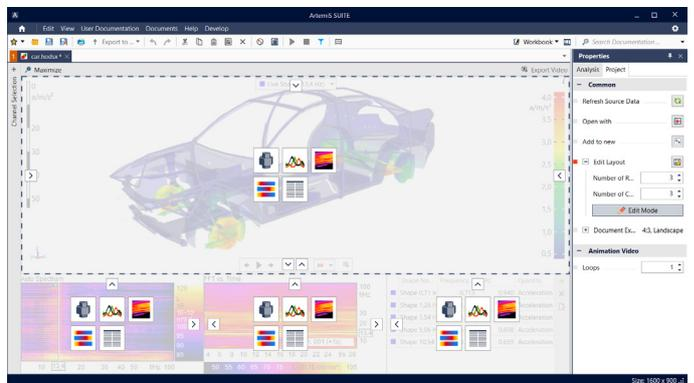
*Edit Mode: The number and contents of the elements can be individually configured and one element selected can be maximized.*
