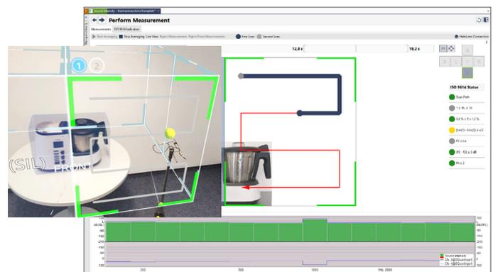
Assistance functions of the Sound Intensity App guide users safely through the measurement procedure. The standard-compliant measurement positions and the measurement progress are automatically visualized via the AR glasses. The app displays measurement results in the measured areas in the form of a sound intensity map including the measured single values.
